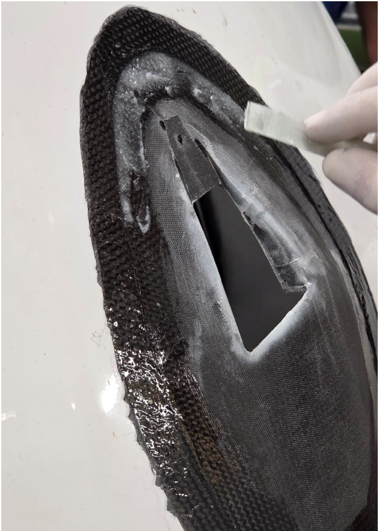
Fig. 18 Filling the transition between the cowling and turbo cooling deflector
