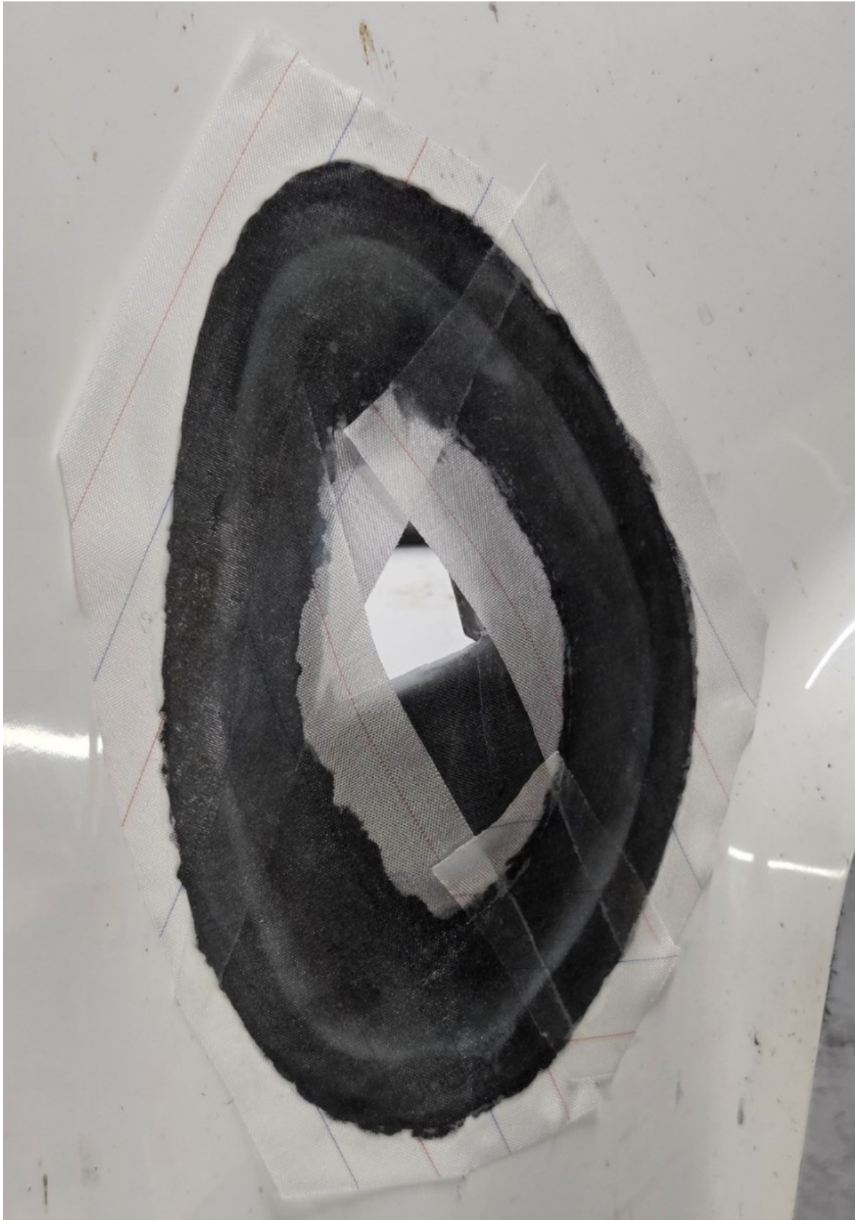
Fig. 20 Peel ply application
