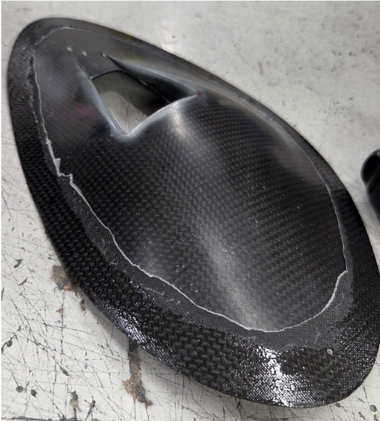
Fig. 13 Wetting the of turbo cooling deflector's bonding surface
