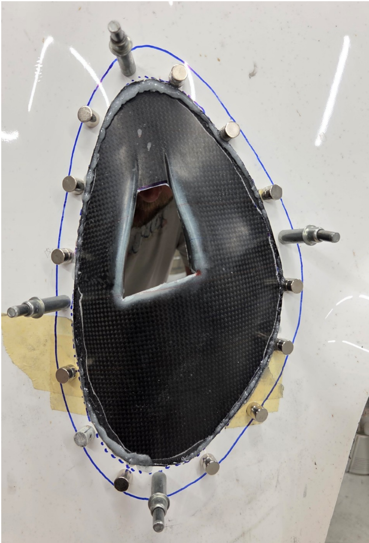
Fig. 16 Positioning and securing the turbo cooling deflector
