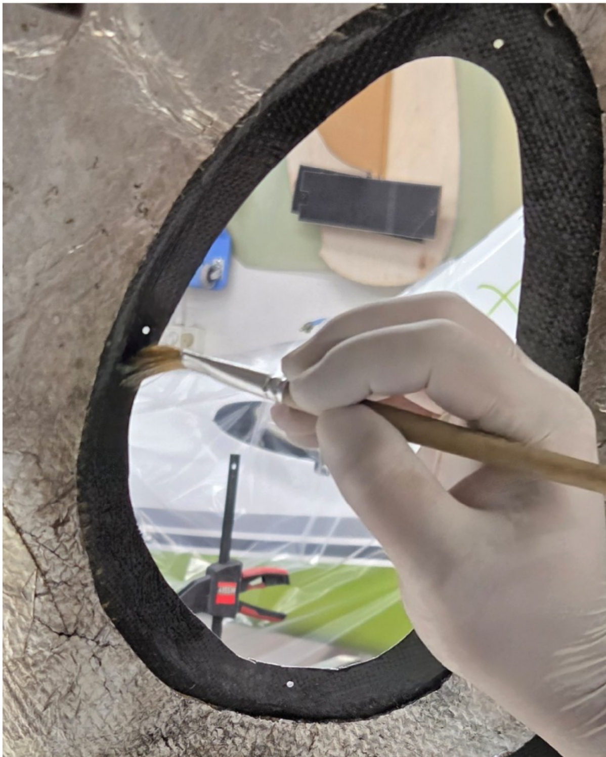
Fig. 14 Wetting of lower engine cowl bonding surface
