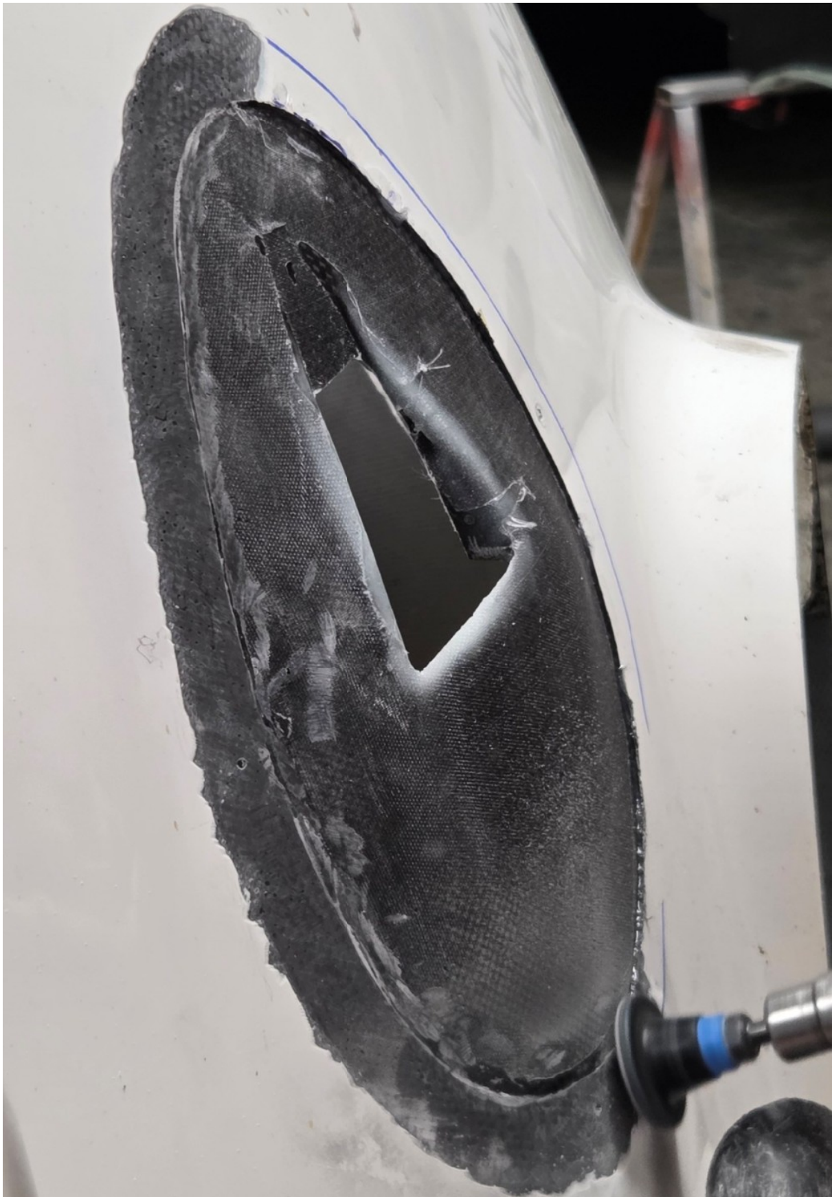
Fig. 17 Grinding smooth transition between the cowling and turbo cooling deflector
