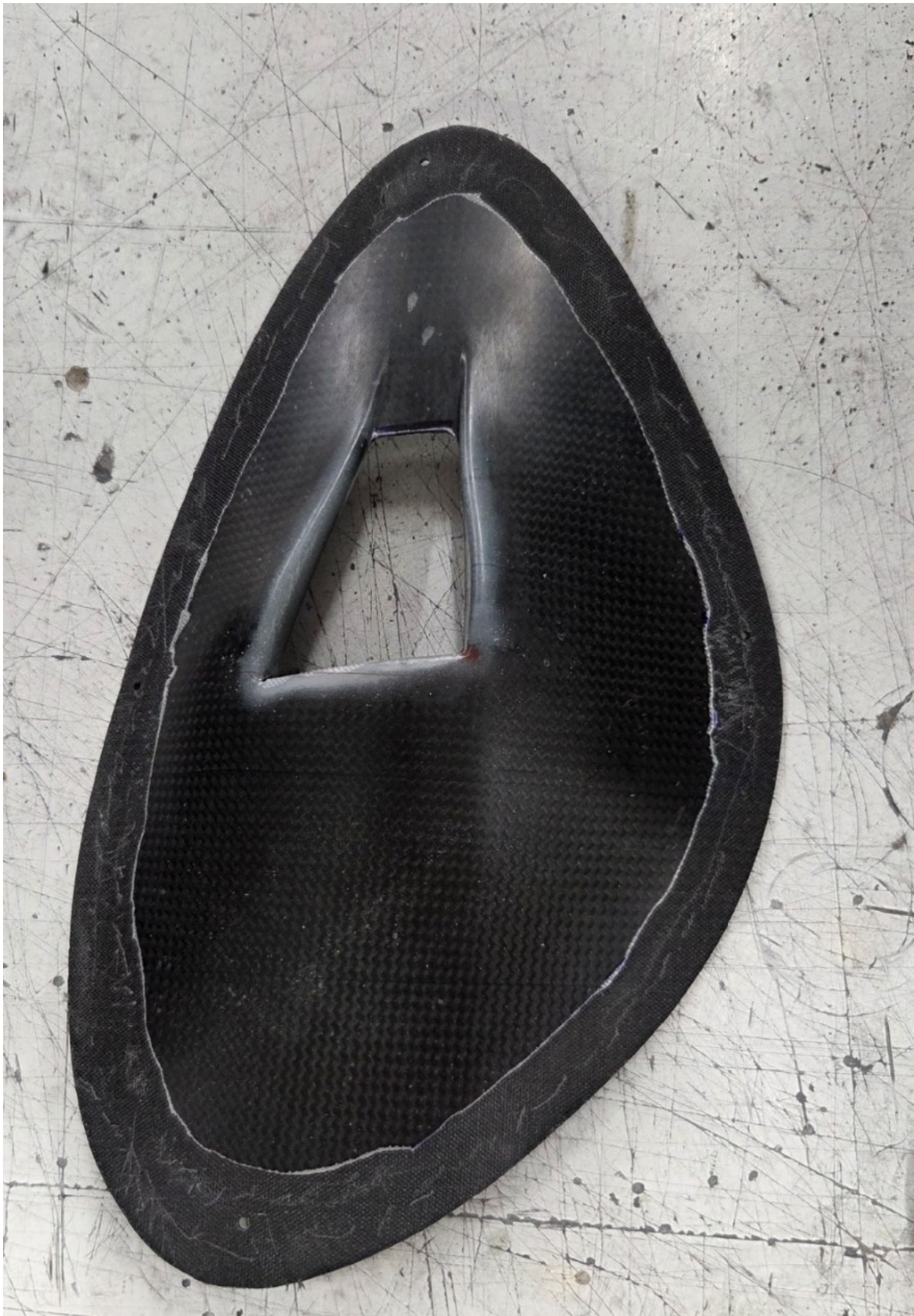
Fig. 10 Peel ply removing
