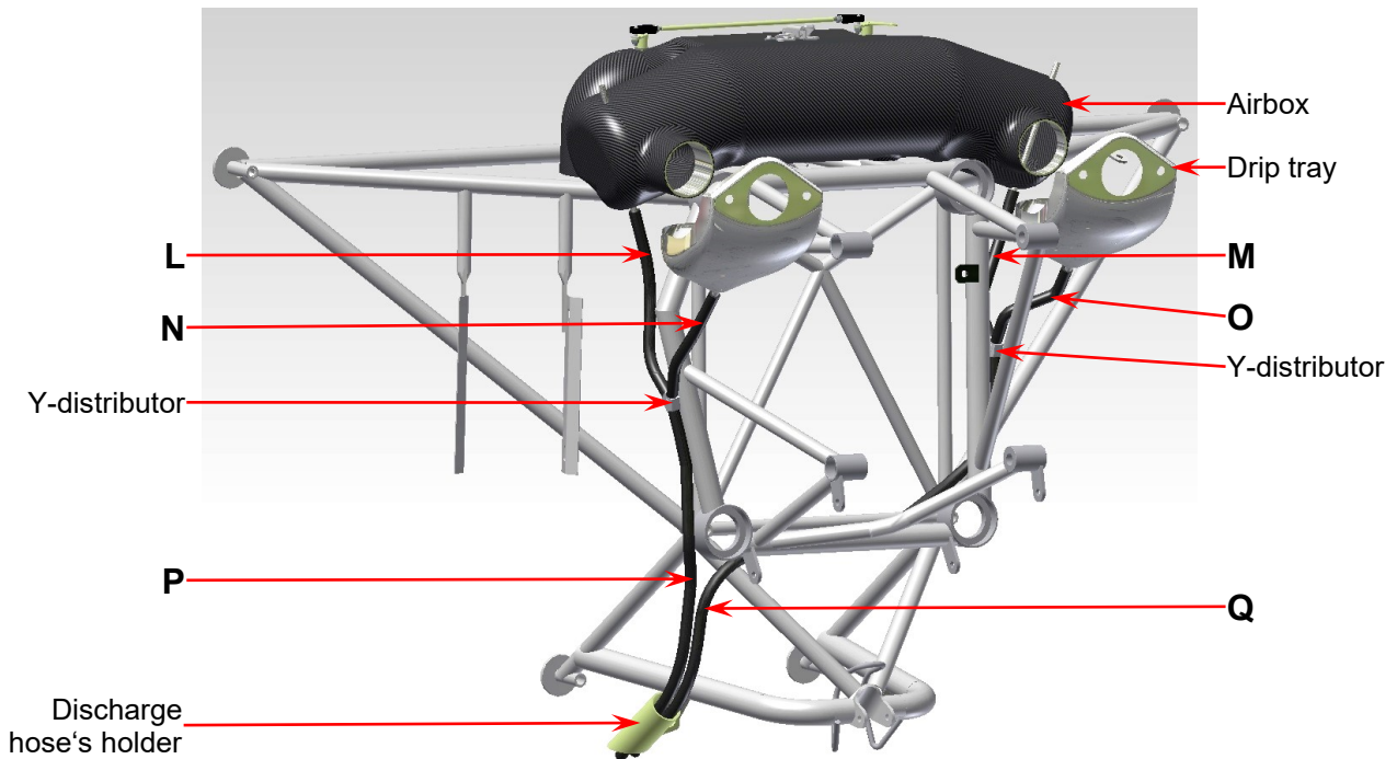
Fig. 2 Disconnecting of drain hoses – Rotax 912, retractable landing gear
