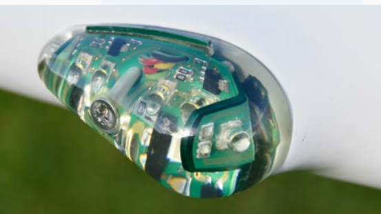
Strobe lights are also nav lights and Flarm sensors
