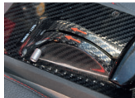
▲ The throttle lever is gated at 100% power, '115%' being full power – 115hp at 5,700rpm
