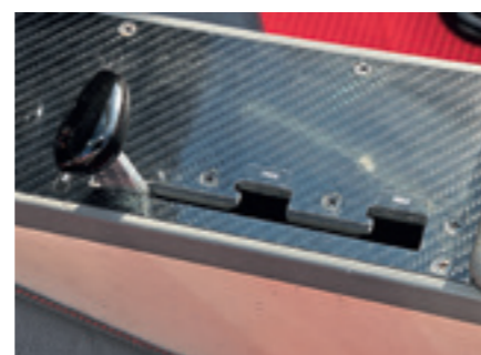
▲ The throttle lever is gated at 100% power, '115%' being full power – 115hp at 5,700rpm
