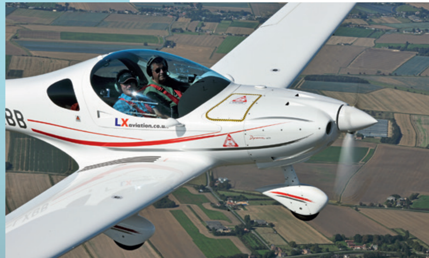
▲ Magnum 601 Emergency Parachute System (EPS) lurks under the panel delineated with a chequered border
