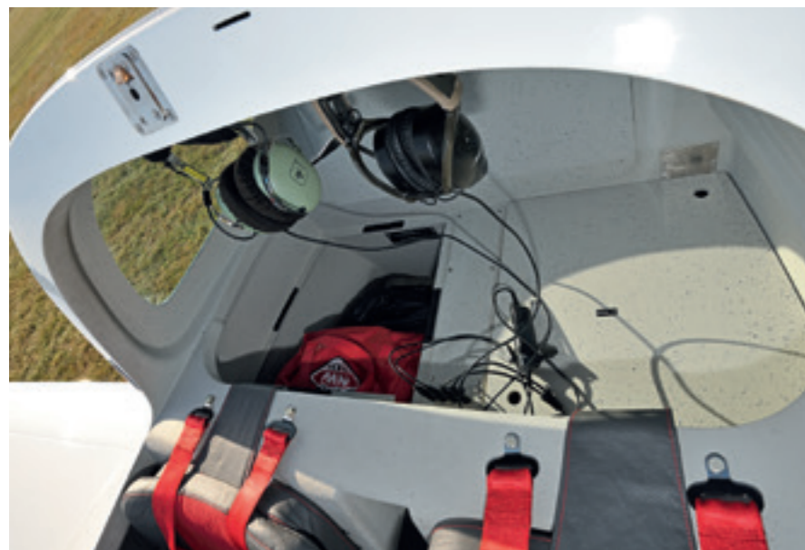
▲ The compartments behind the seats will each take 20kg of baggage, 40kg in total including any item on the shelf
