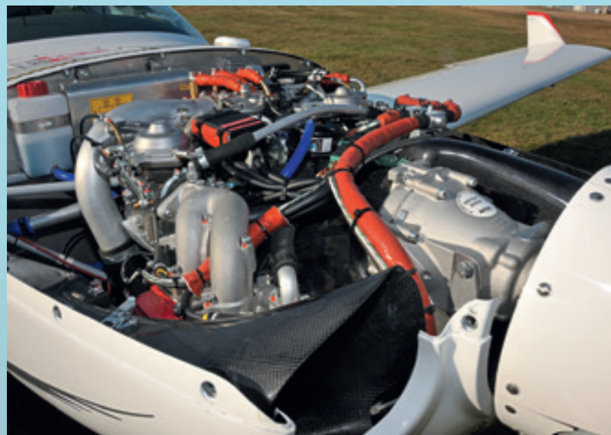
▲ For full access to the engine and inspection of all the hoses, the top cowl can readily be detached
